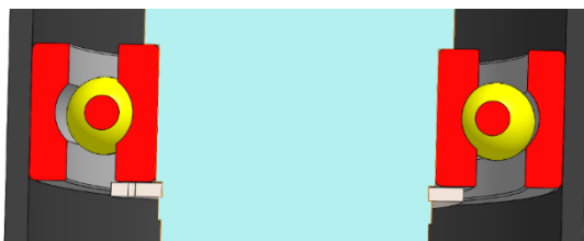
Figure 19 -Output Shaft Non-Locating Bearing
