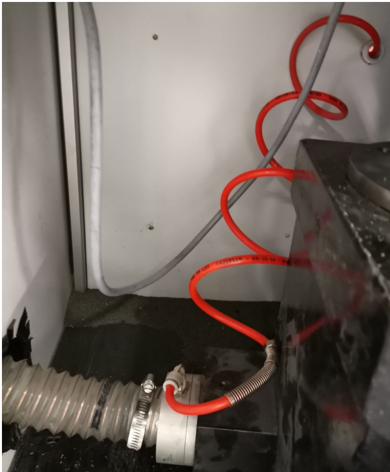
Figure A22 - Compressed Air to Feed Ejector
