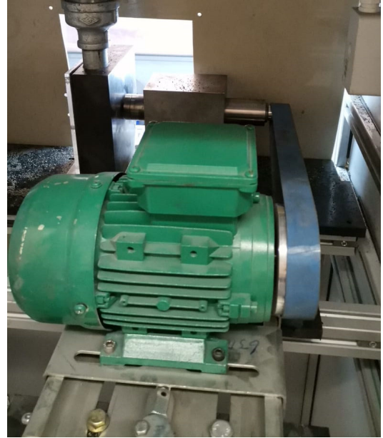
Figure A4 - Fully Assembled Abrasive Discharge System
